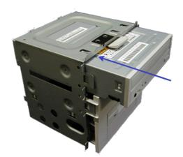
Figure 4 - 10 : Adding a 5.25-inch Device
